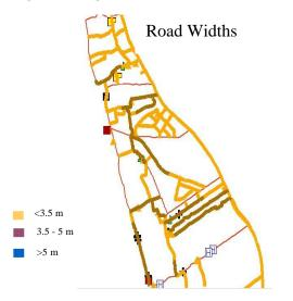
Figure 2: Existing road widths
